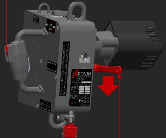
Hold brake fully open by pulling down
