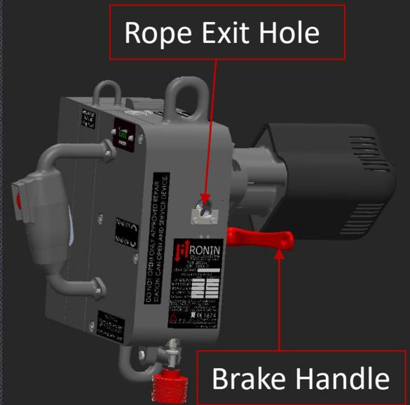
Step 4: Before Ascending turn the red tensioner knob to the clockwise (Right) direction, until hand tight. If you feel the Ronin slipping on the rope during ascending or winching, then stop and turn the red tensioner knob clockwise (Right) 1-2 additional turns, until slipping stops.
